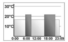
The display will show bars for those heating phases where the set temperature for the period is higher than the saved reduction temperature. With this example no bars for the interval 0:00 to 6:00 are displayed. The bars only appear in the display for the intervals 6:00 to 9:00 and 17:00 to 23:00.
