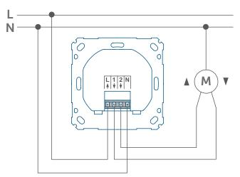
For installation, a neutral conductor is required.
