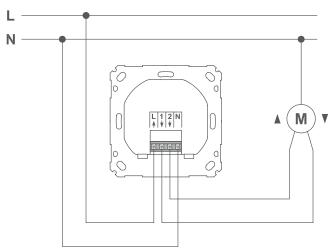
For installation, a neutral conductor is required.
