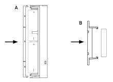
• Then press the electronic unit (A) and the bracket onto the frame and window.
