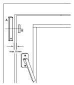
The magnet (B) and electronic unit (A) must be attached at the same level (or as close to the same level as possible) within the designated area. You might need to use the spacers supplied for the magnets (B) to do this.
